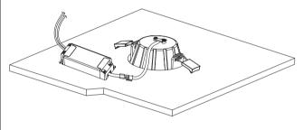
4. Make sure the downlight fixed tightly in ceiling, turn on the power (Fig 1).
