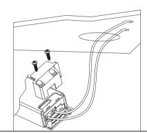
2. Use screw-driver to open the driver terminal cover, feed the main AC wire L. N. in terminal block respectively, then fix the cover back.
