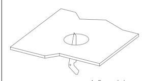
1. Open a hole according to the cutout size of led downlight.
